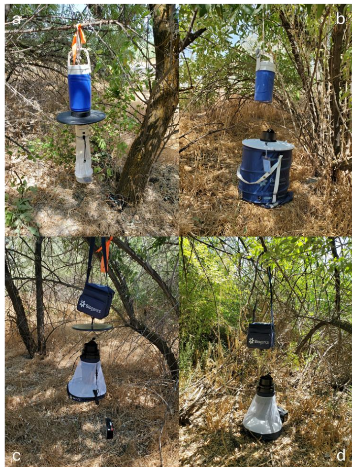
Figure 9 (a) CDC, (b) BGSENT, (c) ProCDC, and (d) ProSENT trap configurations under field conditions.
